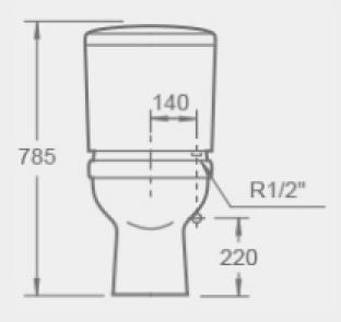
Universal outlet pan (P-trap and S-trap) UF seat cover,
